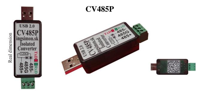
CV485P is the converter between USB and RS485 with optoisolated communication. Power for optocupler and for IC is solved via DCDC converter.
